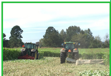
Termination of okra using no-till options: a roller-crimper (left) and hay mower (right)
